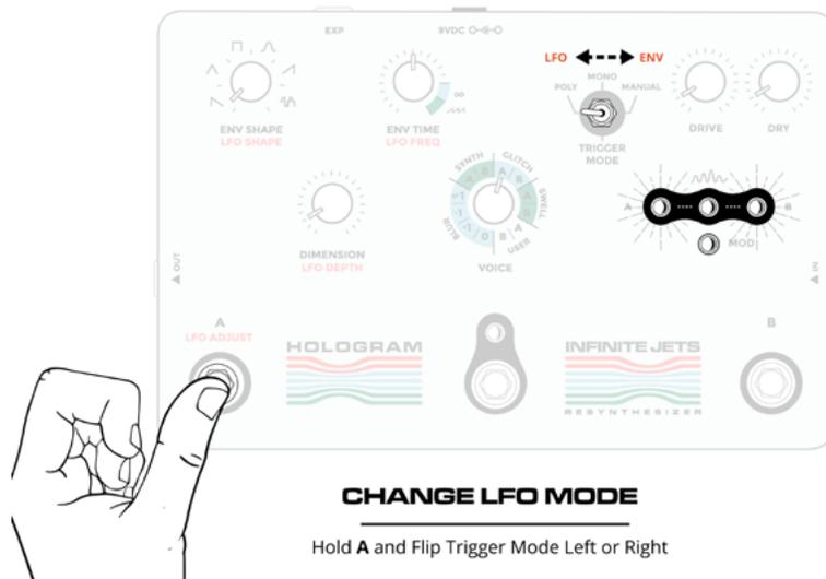
To switch between **LFO** and **Envelope Generator**, hold **Footswitch A** and flip the **Trigger Mode** toggle switch left for **LFO** operation or right for **Envelope Generator** operation.
