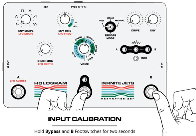
In order for Infinite Jets to accurately track the dynamics of your playing, it's necessary to calibrate the pedal to each new instrument that you will be using. It only takes a few seconds and can be done mid set or even mid song.
