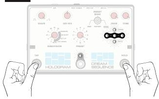
Hold both outside switches again for two seconds, or press Bypass to cancel. Indicator lights will flash green when completed.
